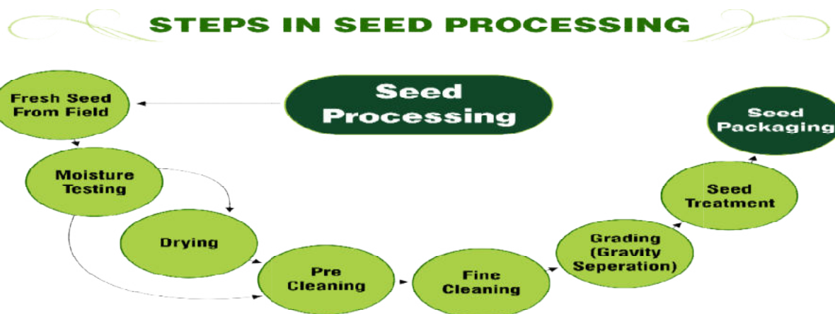
Fig-1.: Steps involved in oilseeds and pulses seeds processing
