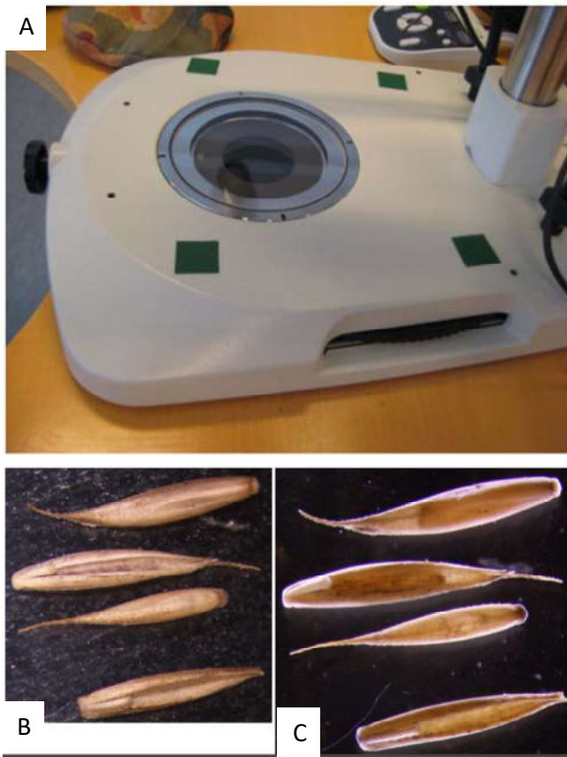
Fig.3. (a). LED transmitted light mounted microscope (b). As seen in microscope with light above (c). As seen in microscope with LED transmitted light from below
