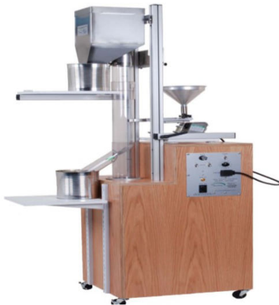
Fig.4 Continuous flowing blower
